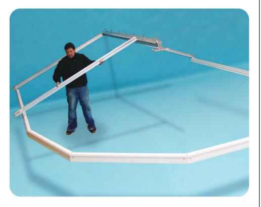
Now working left to right viewed from outside, fit all the side transoms. Locate the pin of each transom into the ring beam, then aligning the holes at the top with those pre-drilled on the ridge. Now fix at the top and the bottom using the short wide self tapping screws provided. Repeat process until all the transoms along each side of the roof are in position.
